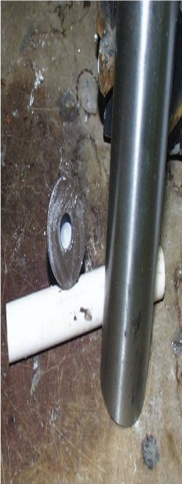
Bottom of carbide (showing countersunk hole) and shaft
