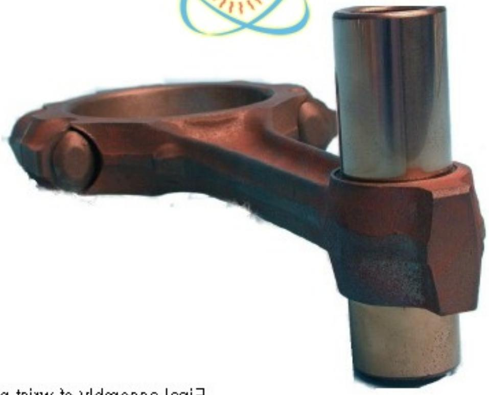
Final assembly of wrist pin & rod
