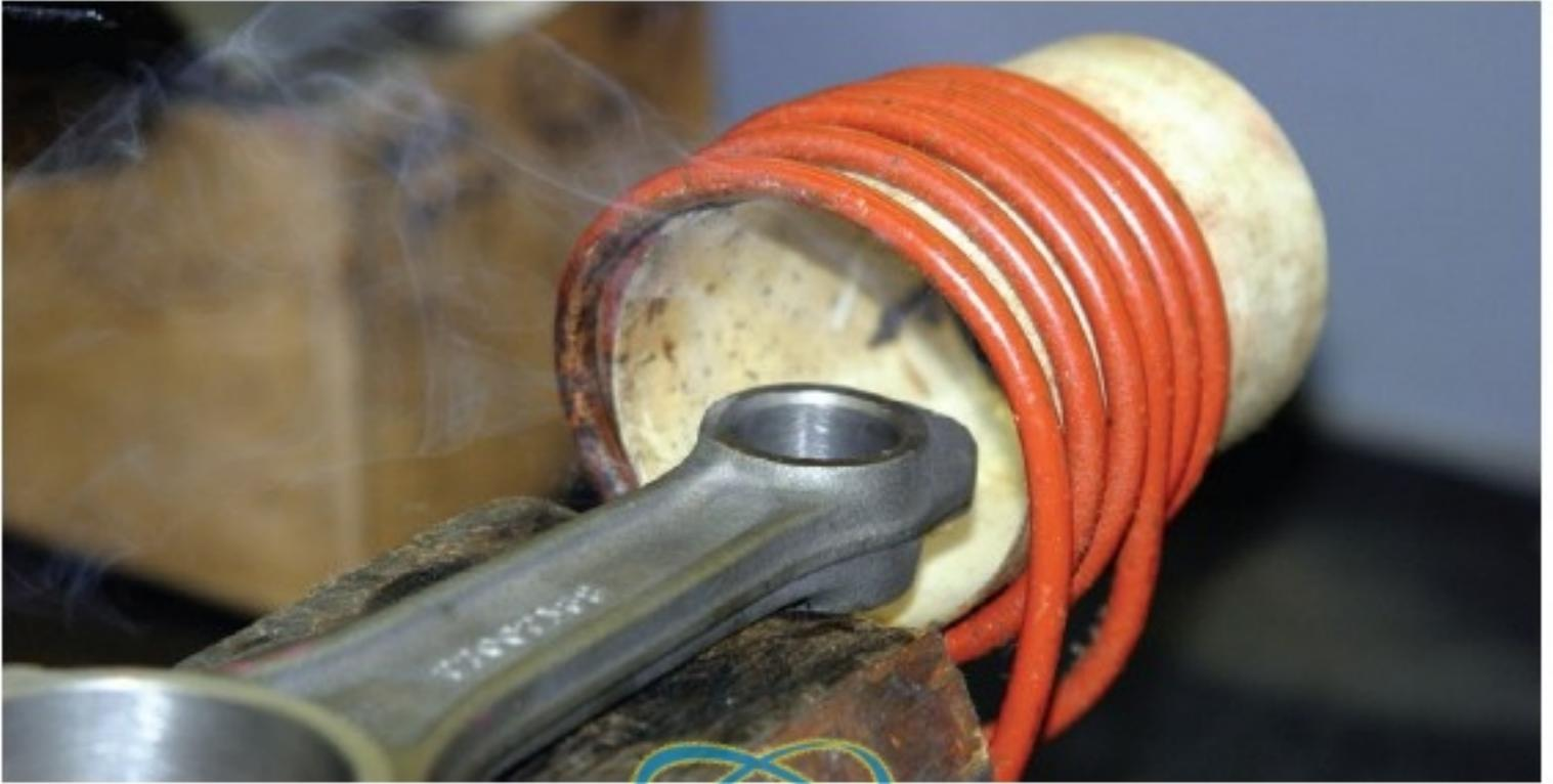
Coil is perpendicular to the axis of the bore when heating the knuckle
