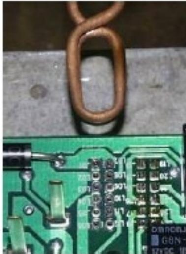
**Twelve preforms in place for soldering**
