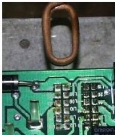
**Completed soldering of the 12 post**
